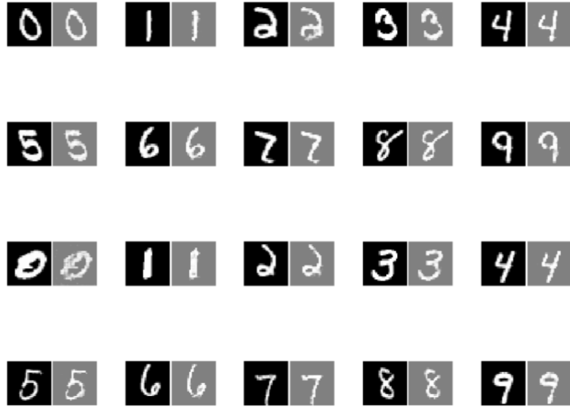
Figure 4. Examples of real inputs (left) and fake outputs (right) for the SegNet autoencoder. Compared to the VAE, the SegNet is less confused about the structure of the input images. However, the two channel output results in an average of the binary masks which gives a gray image.
