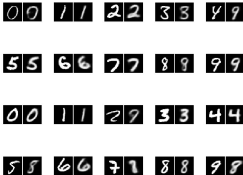
Figure 2. Examples of real inputs (left) and fake outputs (right) for the VAE. The pairs demonstrate examples where the VAE performs well and where it does not, noticeably a ‘9’ that becomes an ‘8’ and a ‘4’ that becomes a ‘9’.
